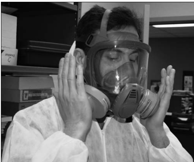
Negative-pressure seal check
