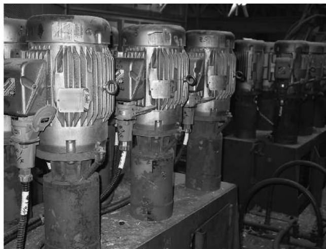
Flash protection is designed into this disconnect switch/plug
